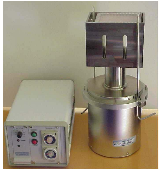
Sonication of microtiter plates: generator, transducer with sonotrode and on the top the microtiter plate
