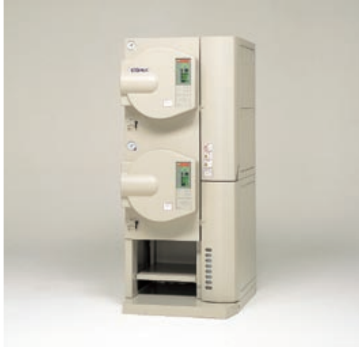
Photo 1 TABAI HAST CHAMBER Model: EHS-411MD (Dual vessel)
