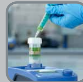
STEP 9 If required the sample can be extracted for analysis with a syringe through the pierceable membrane of the tube lid.
