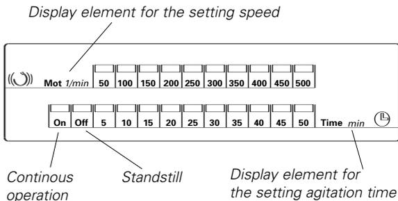
The basic model of the device can be used in continuous or timed mode depending on the option you select. The right turn button is used to make the setting.
