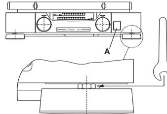
To prevent the foot of the device from coming loose by itself, hold down the foot with one hand and tighten the opposite hexagonal nut with the other hand until it is finger tight.
